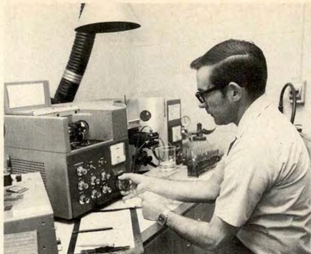
479 FMS SOAP laboratory supervisor, William C. Moffat, calibrates Perkins-Elmer 303 unit in preparation for the day's analysis.
