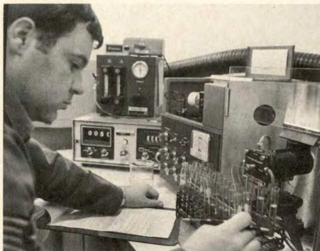
J79 engine oil samples are tested for iron content by SSgt Raymond B. Borm.
